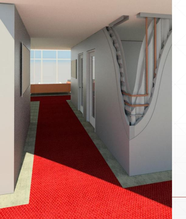
Studless construction – just upper track, lower track, and splines.
